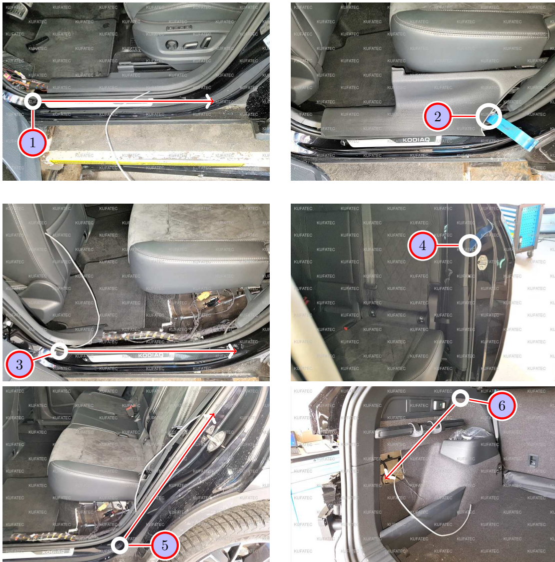
Figure 7: Cable routing to the sound generator
